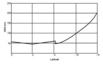
Figure 5. SSR-1 Ground Sample Distance (GSD) as a function of latitude.
