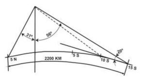
Figure 3. SSR-1 viewing geometry
