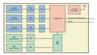
Figure 4. Payload block Diagram
