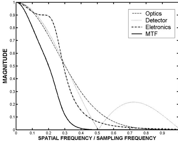
Figure 1. Modulation Transfer Function model components.
