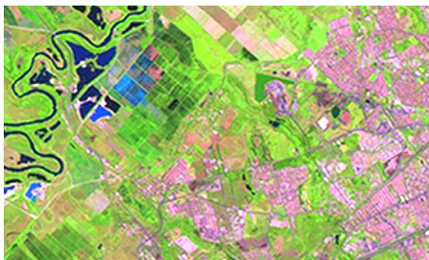
Figure 4. Restored ETM+ image – Color composite 3B4G5R with pixel size of 10 m.
