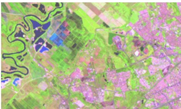
Figure 3. ETM+ interpolated image– Color composite 3B4G5R with pixel size of 10 m.
