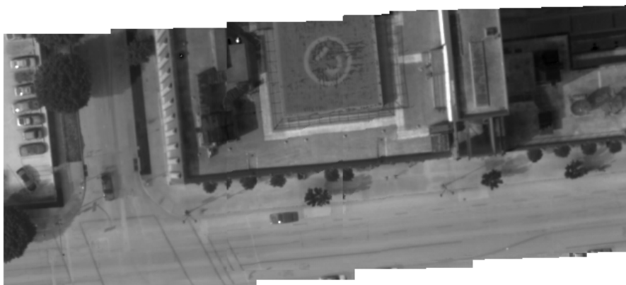
Fig. 23 - Mosaic of a aerial IR video sequence mosaic: 107 images, 256x256 pixels, generated in 20 seconds.
