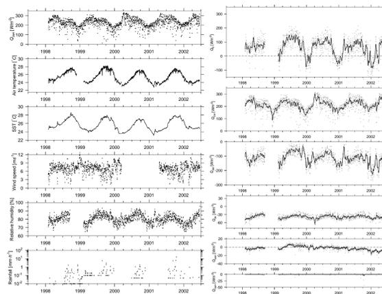
FIGURE 3: Variables measured from buoy 15°N 38°W (left) and surface heat flux components.
