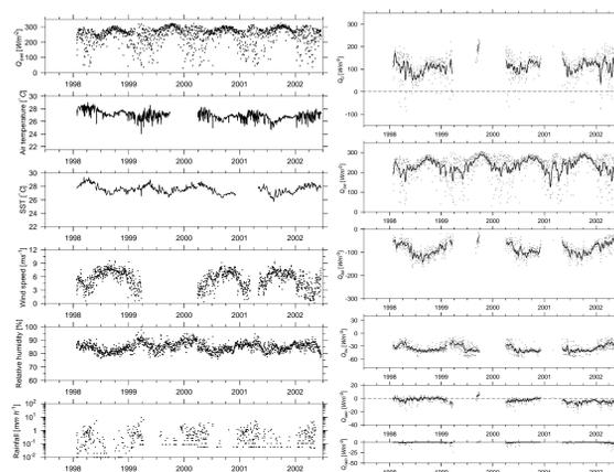
FIGURE 4: Variables measured from buoy 00° 35°W (left) and surface heat flux components.
