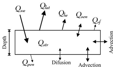
FIGURE 2: Heat fluxes components of mixed layer.
