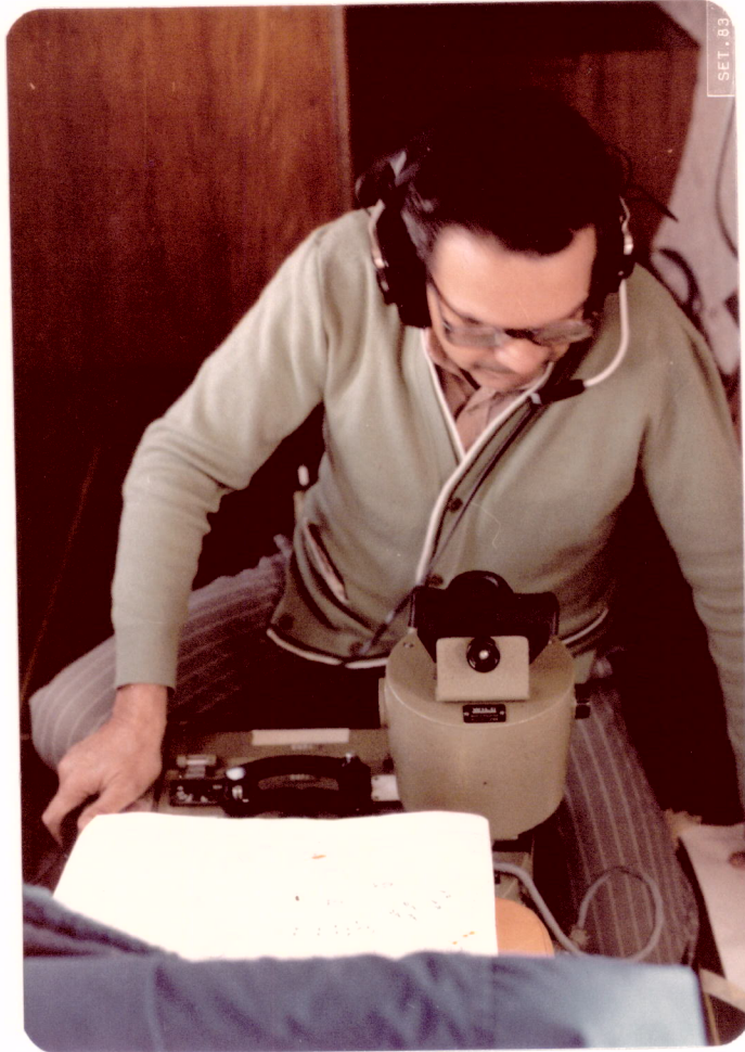
Fig. 11 - Phototechnician making final adjustments on RC-10 Camera prior to photographing a target.
