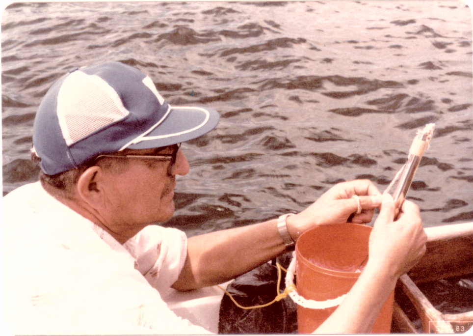
Fig. 4 - Measurement of surface water temperature using a calibrated thermometer.
