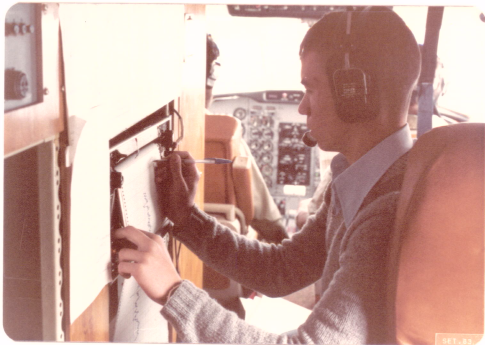
Fig. 13 - Observer marking the time of passage over a landmark seen by the technician using the RC-10 Camera.
