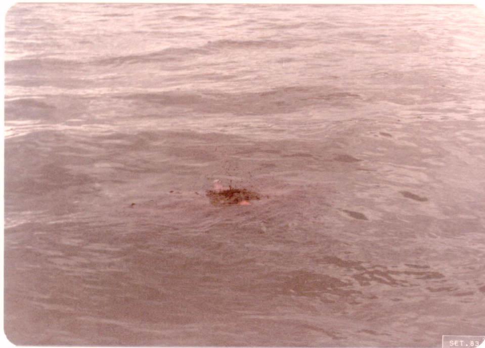
Fig. 7 - Photograph taken at the instant a dye filled balloon is broken using a pellet gun.
