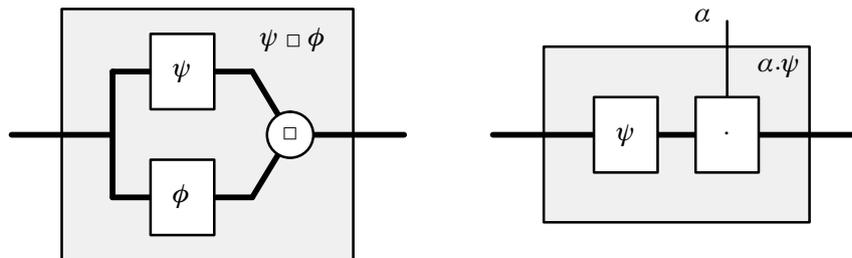
Fig. 3.9 – Internal and external binary operations on image operators.
