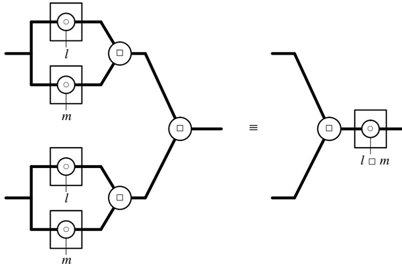
Fig. 3.13 – Two equivalent implementations when the luts are morphisms.
