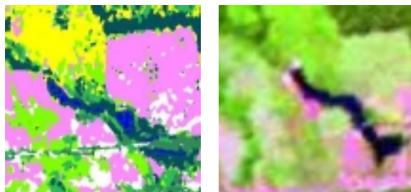
Fig.3. Zoom from area 2, illustrating the correct classification of a new regeneration area and the confusion between bare soil, pasture and crops.
